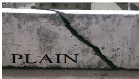
Fig. 5. The formation of crack in plain and fiber beams
